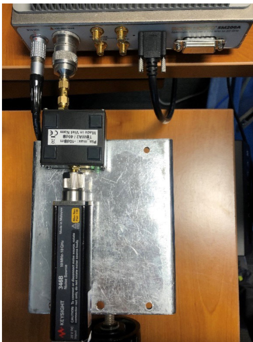
Figure 12: Keysight 346B noise source connected to TekBox TBWA 40 dB Wideband Amplifier (DUT) connected to Signal Hound SM200A spectrum analyzer in DUT measurement step.
