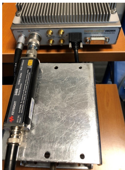
Figure 10: Keysight 346B noise source connected to Signal Hound SM200A spectrum analyzer in calibration step.
