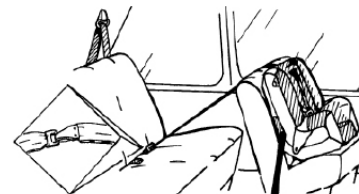
A CR installed in the second row of a van, tethered to a third-row latchplate.
