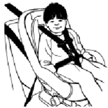
Big kids who ride in a CR with a harness are safer when the CR is tethered. Consider all ways to limit head excursion, especially if tethering in the typical manner is not possible.
