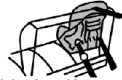
Labels on forward-facing CRs made after February 2015 must appear near a diagram like this and state, "Do not install by this method for a child weighing more than XX pounds."
